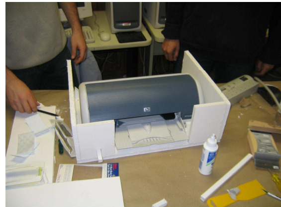
Figure 3: A photograph showing the construction of our embodied printer device.
